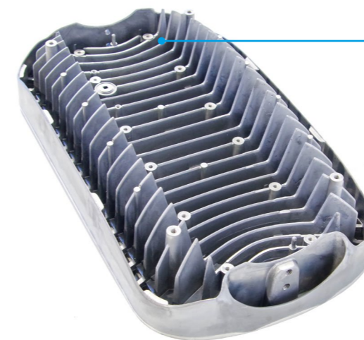
3 DIE-CAST BODY AFTER MACHINING ON BROTHER 630 MACHINE TOOL
