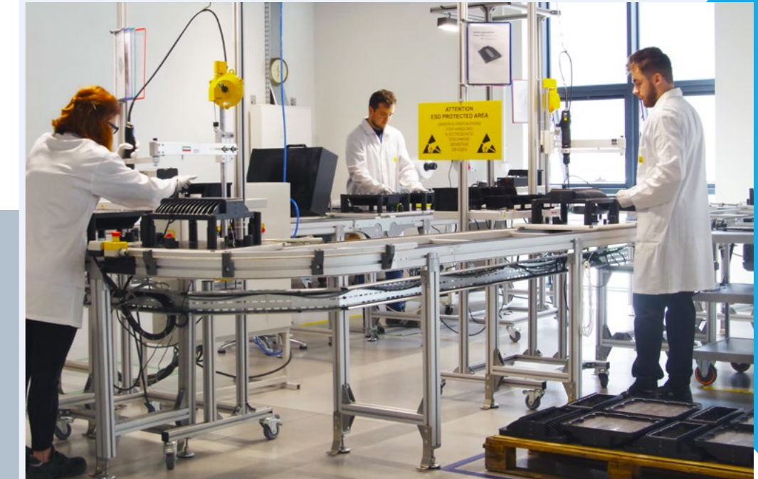
Semi-automated LED lighting assembly line
